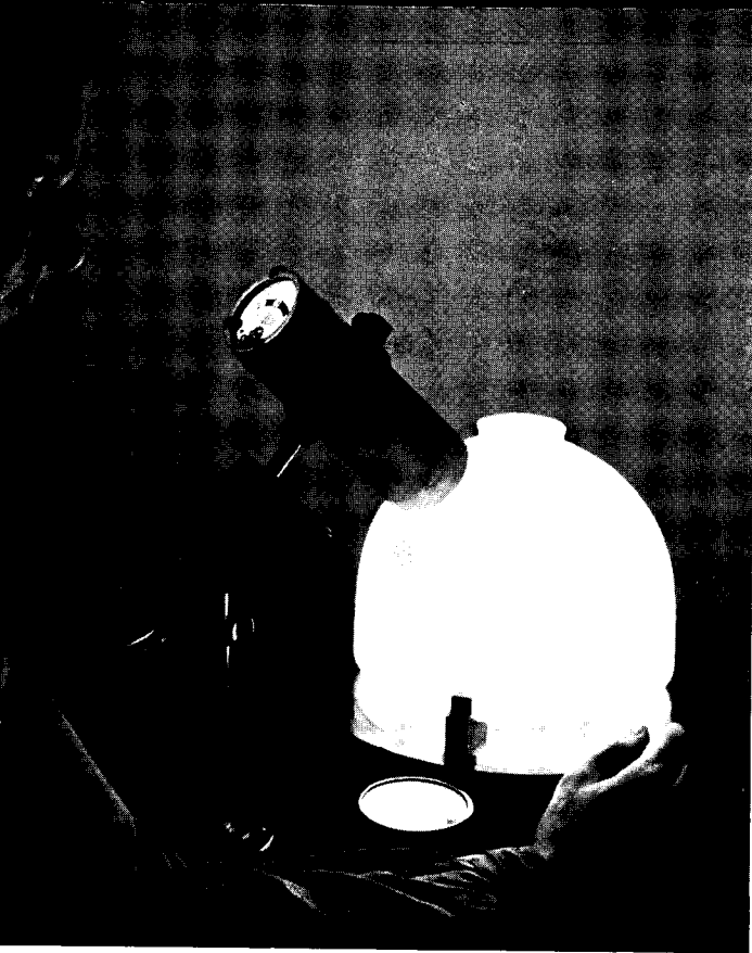
Measuring performance of light diffuser in laboratory
