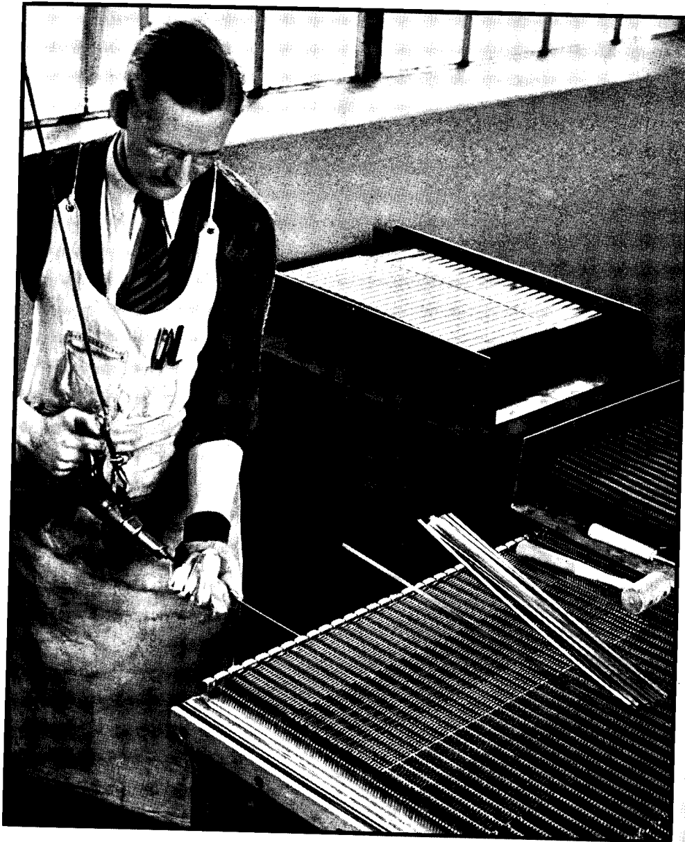
Assembly of UNI-FLO Grille Core with Directional Diffusing Fins on Specially Designed Assembly Table
