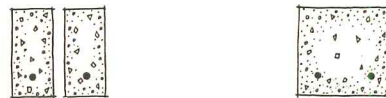
Pre-cast concrete lintels, requiring steel only in the pencil rod reinforcing, may be used in place of steel lintels, with considerable metal saving
