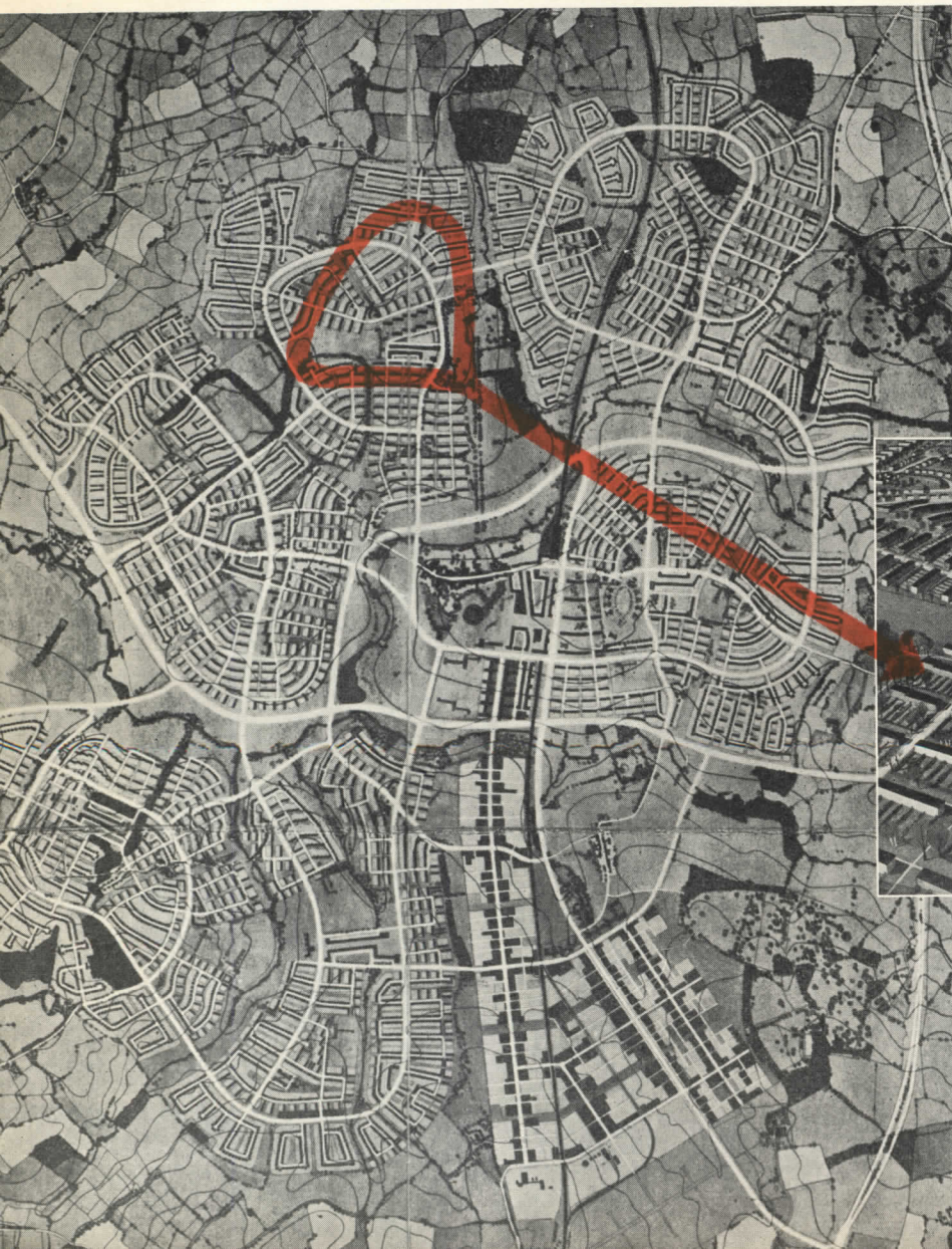
LEFT: Aerial view of the proposed satellite town of ONGAR. It is planned to contain six distinct neighborhoods, each accommodating about 10,000 people, and each roughly enclosed by a main artery or loop road
