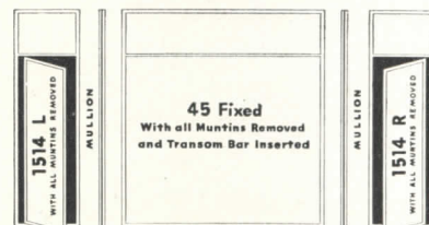
Remove all muntins and insert transom bar as illustrated. Combine windows with standard mullions.
