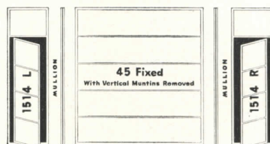
Remove vertical muntins from Ceco stock casement 45-Fixed. Combine windows with standard mullions.
