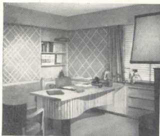
OFFICES. Birch Weldwood combined with wallpaper. Valance is decorative and practical — it conceals drape and blind attachments, and provides space for indirect lighting fixtures at the same time.
