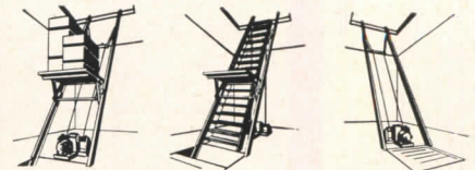
Stairlevayor, a motorized lift designed for use in open spaces or over stairways
