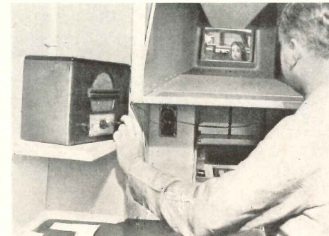
Above: Mercantile-Commerce Bank & Trust Co., St. Louis, Mo. Curb teller gives drive-up service where space is unavailable for window. Deposit placed in unit is lowered to teller's booth below sidewalk. Mirror system and two-way speaker permit customer and teller to see and converse with each other
