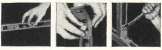
Insert nut into slotted channel Locate fitting and nut Tighten bolt — it's done
