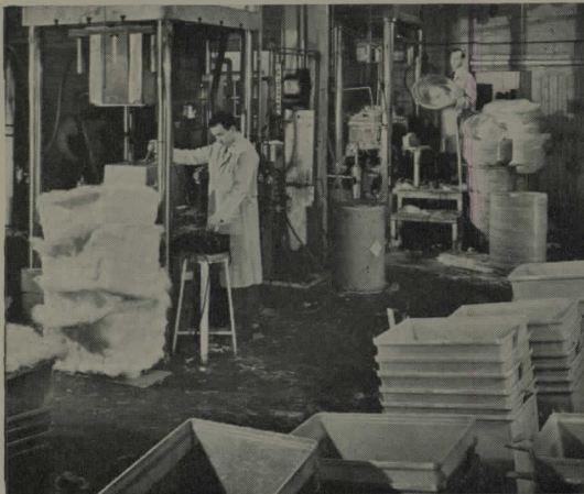
4. preformed fibrous glass mats for the boxes in the foreground are stacked near one of the molding presses; more complicated parts with spiralled grooves can be seen in the background. 5. large corrugated sheets of reinforced plastic form decorative partition
