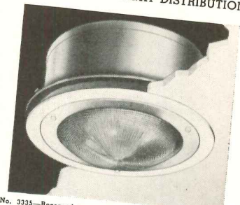
No. 3335—Recessed type. Holophane Prismatic Glass Refractor provides a widespread symmetrical pattern light distribution. Spacing up to 2.0 times the mounting height above surface to be lighted provides uniform illumination.
