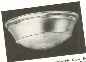
No. 3353—Surface type. Holophane Prismatic Glass Refractor provides an Asymmetric (corridor-type) light distribution. Spacing up to 2.5 times the mounting height above the floor provides uniform floor illumination.
