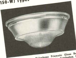
No. 3353—Surface type. Holophane Prismatic Glass Refractor provides an Asymmetric (corridor-type) light distribution. Spacing up to 2.5 times the mounting height above the floor provides uniform floor illumination.
