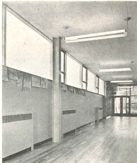
Top of page, cafeteria which is also multi-purpose room. Above, single-loaded corridor. In both, note the exposed, low-brightness fluorescent lighting. Below, stair hall
