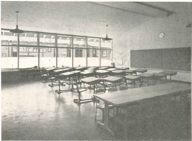
Below, two new classrooms, now joined as multi-purpose room, can be partitioned off. Interior walls, wallboard; ceilings acoustic tile; exterior walls stucco
