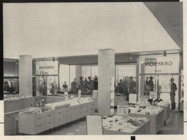
\*Neo-Ray Louvred Ceiling was chosen for good even lighting and a minimum of maintenance. The 3" x 3" opening is architecturally good in scale for large rooms.
