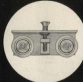
Tandem radial ball bearing nylon rollers that roll flush in line contact on a flat trackless threshold are fully adjustable, an important feature allowing a full true alignment of door with jamb.
