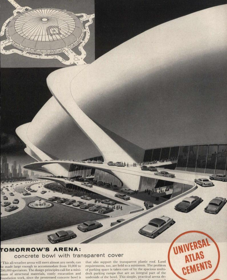
"This all-weather arena will meet almost any needs, can be made large enough to accommodate from 10,000 to 200,000 spectators. The design principles call for a minimum of structural materials, costly excavation and foundation work, since the prestressed concrete bowl is bound together into a unified structure by the steel cables
