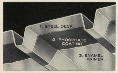
TOUGH NEW FINISH STAYS ON. A thin phosphate coating, applied to clean sheets, protects metal and prepares it for painting. Then, rust-preventive battleship grey enamel is "flow coated" over the metal for an even finish. Baked on at 400° F. for 20 minutes, this durable flint-hard enamel adheres tightly, resists abrasion and chemical corrosion, protects metal years longer.
