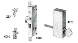
The 1848 Sliding Wall Deadlock shown above measures only 3%," x 1%" x 1%", has a collapsible bolt for protection of door and lock, and operates with positive "feel appeal". To compensate for possible misalignment of door and jamb, bolt projection can be adjusted a full %" by simply turning a screw in the lock face. The 4025 cylinder group is a clean-lined outside pull, offering key control that can be keyed-in with most popular cylinder systems.
