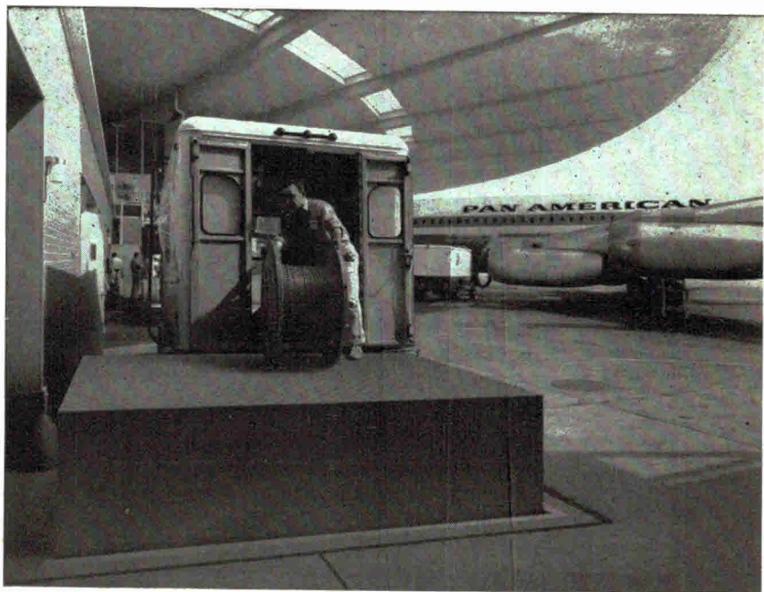
Rotary Levelator Lift (6,000 lb. capacity) raises freight to truck bed height for fast transfer to Pan American plane.
