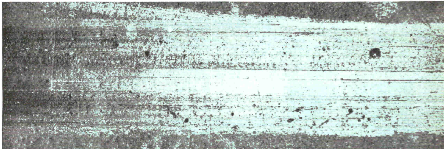
HERE YOU SEE THE LAPIDOLITH treated concrete after 500 strokes. Note that even under six magnifications the surface appears unbroken, with total wear being measured at only 0.0003 inch! The equivalent of 1/3 of 1 mil! Particles of metal may be seen imbedded in surface of the concrete.
