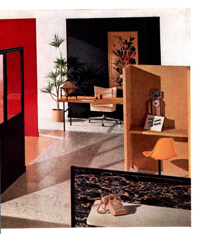
aptability, these walls offer many er important advantages. They go fast. They are only 1¾" thick, yet y are sturdy in appearance and rdy in service. They can be easily 1 quickly moved, re-using every ce of material. They have an inhustible core. They have asbessheet facings. They have steel ming. They meet most fire codes. I-M High Wall panels fit into tal floor and ceiling channels. se and cornice snap on, to com-
