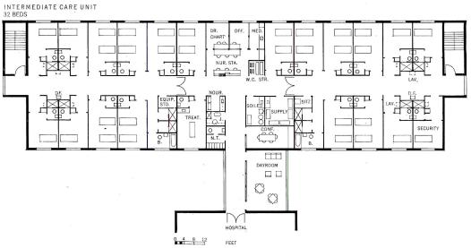
Figure 2. Single-Corridor Patient Care Floor. One patient care unit, utilizing carts for transportation of supplies and food trays to and from unit. This type of unit can be used for additions to existing hospitals, or in modified form wherever single-corridor units are indicated
