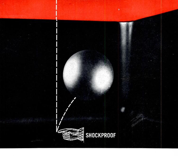
**DURCON® LABORATORY SINKS** can take it. As shown above, our quality control engineers drop a 3-lb. steel ball into Durcon sinks from heights of 6 to 9 feet. These tests prove Durcon resists impact blows far greater than those encountered in normal lab service.
