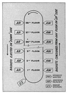
"Magnetic memory" control system has no moving parts, no levers, no between-station wiring . . . nothing to wear out. Diagram shows how address "writers" and "readers" are located between the building's 28 floors. If you are planning a multi-story building where mail distribution can be a problem, get the full details now on fast and efficient Recordlift!
