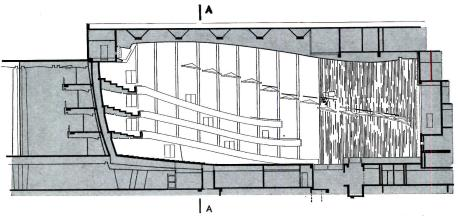
FIG. 2: Longitudinal section of Philharmonic Hall along the centerline. Total seating capacity is 2,644 divided as follows: orchestra (main floor)—1,384; loge (first balcony) -392; first terrace-454; second terrace-414
