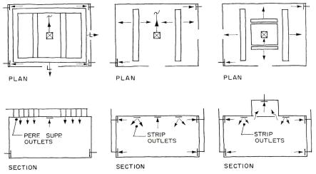
Three good, wide-area, air supply arrangements for operating rooms. Note low exhaust at corners and ceiling vent for heat relief over operating table lights
