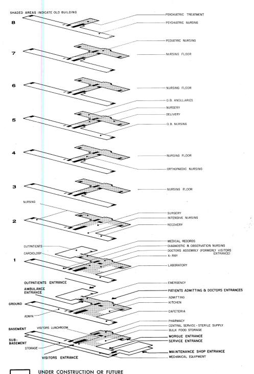
The isometric schematic shown above indicates the old main hospital building and the new additions. The major functions of the building are shown in a manner indicating their prime relationships to each other, as these now exist. The older portions of the hospital have been completely renovated and related to present hospital functions.
