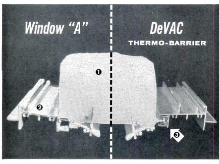
Dry ice is used at -240° to demonstrate conductivity of two aluminum window sections.
