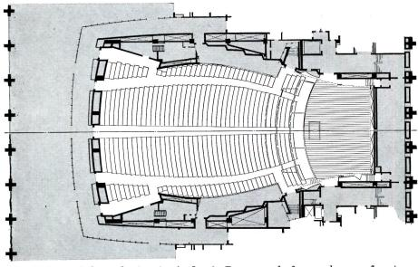
FIG. 3: Plan of the orchestra (main floor). By removal of several rows of seats on the main floor, the stage depth can be increased from its basic depth of 40 ft at centerline to either 48 or 56.5 ft
