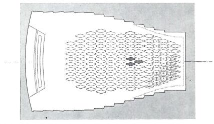
FIG. 6: Reflected ceiling plan showing the lower layer of sound-reflecting panels. These panels are made of hard-white finish plaster over metal lath and colored by gold leaf. Three panels in the center, however, are wire mesh only so that they will be acoustically transparent to the loudspeakers behind them. The loudspeakers are not used by symphonic orchestras, but only as required for dance bands, popular vocalists, public speakers, etc.
