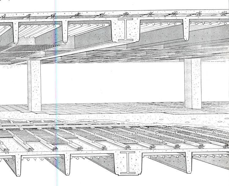
The plenum can be varied in height to meet any capacity requirement. Baffles zone air to desired areas. Adjustable supports assure level finish floor, compensating for dead load deflection and irregularities in structural slab.
