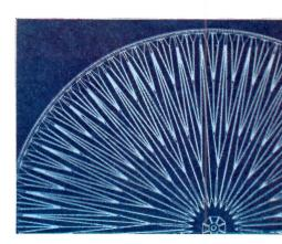
Intricate design pattern of roof is shown in this detail sketch. The webs of the interlacing folded plate segments of concrete are as thin as 3½ inches. The center of the dome is 128 feet above the floor.
