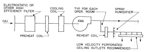
Schematic of a conventional system for operating suite. This arrangement is low in cost and requires less space than modifications shown below. Needs regular maintenance to keep algae under control
