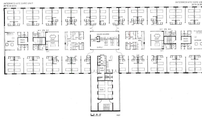
Figure 1. Double-Corridor Patient Care Floor. Consists of one 30-bed and one 32-bed unit, and utilizes centrally located mechanical conveyors for handling of supplies and food tray services
