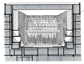
FIG. 5: Transverse section A-A. Note rectangular cross-section of the hall
