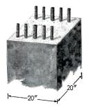
2 #11+8 #10; /.s=13.28 sq. in. f'c=3000 psi fy=60,000 psi Saving Over Basic Design Steel=15%
