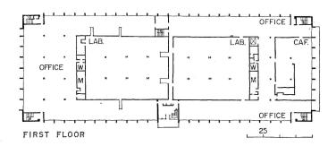
Great flexibility for both office and lab spaces has been provided to make the building adaptable to the various product development projects which may arise. All mechanical, heating, and electrical services are planned to permit partitions to be moved at will on a 2-ft module. The two main floors and the service floor contain 163,000 sq ft of space. Offices are enclosed by a combination of movable glass and steel partitions to provide light or wall space where needed.
