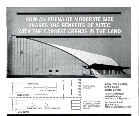
Altec's functional simplicity made it possible for the moderately-sized civic arena in Sioux Falls, population 65,000, to enjoy sound reproduction equal in quality to the largest structures of its type. Thanks to Altec high efficiency speakers, only *two* power amplifiers — both of medium power output — are used. Within the arena, only four Altec multicell horns provide clear voice reinforcement regardless of high ambient noise levels.
