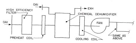
More elaborate system requires additional ductwork and louvers but keeps algae and micro-organisms to a minimum with some increase in operating cost
