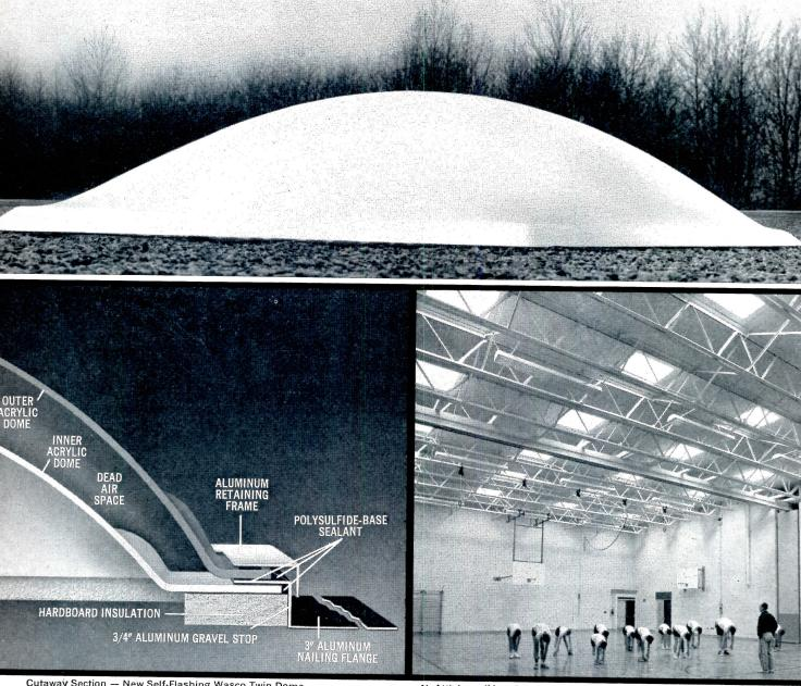
Cutaway Section — New Self-Flashing Wasco Twin Dome
