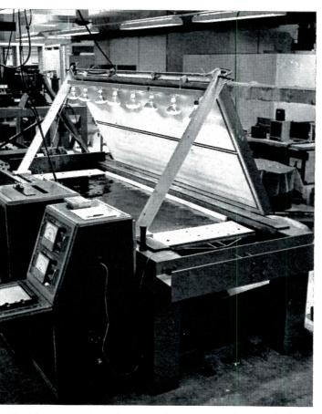
Heat lamps are turned on to raise a test specimen of built-up roofing over deck structure to temperature around  $150~\mathrm{F}$
