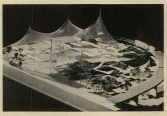
German Pavilion: The German Pavilion will feature a giant steel mesh canopy supported by trussed masts from which a skin of heavy translucent fabric will be suspended, covering a series of terraced exhibits. Weather permitting, the interior of the \$10 million pavilion will be kept open from all sides. Architects are Professors Frei Otto and Rolf Gutbrod. Canadian associates are O. Tarnowski and George F. Eber.
