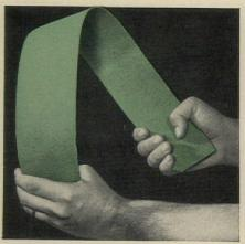
**Permanent flexibility.** Traffic Topping is resilient... expands and contracts without cracking even at temperatures as high as  $300^{\circ}$ F, as low as  $-65^{\circ}$ F.
