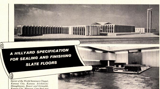
Shaughnessy, Bower and Grimaldi, Kansas City, Missouri. Cem-Seal was applied for protection during construction and installation of pews. (In progress above). After pews were installed, two thin coats of Super Hil-Brite carnauba wax provides the wearing surface.
