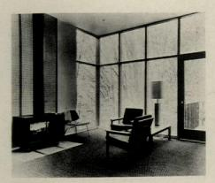
FIREPLACE / The simple styling of this unit fits a variety of interior decorating schemes. The fireplace may be used as a free-standing floor unit or with wall brackets for mid-wall suspension. Models may have top-mounted vertical chimneys or hidden back flues and, although listed by Underwriters' Laboratories as solid fuel units, are adaptable to gas-log conversion with hearth openings to 40 in. " Condon-King Company, Inc., Lynnwood, Wash.
