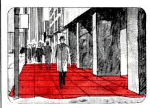
[Snow Melting] Chromalox Electric Heater Mats and MI Heating Cable are embedded in concrete or asphalt sidewalks, driveways, ramps and steps to keep surface areas free of ice and snow. They eliminate manual labor and related costly agents such as salt, cinders and chemicals which often are tracked indoors to stain rugs and floors.
