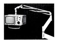
HOSPITAL TELEVISION SYSTEM / A fully transistorized electronic system provides both audio and video intercommunication in addition to furnishing individualized TV entertainment for patients. The system requires only a single coaxial wire. A balanced arm keeps the miniature set at the correct viewing position and within the patient's reach so that he can make all set adjustments without the aid of a nurse.
