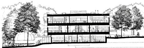
The three-story building is set on a sloping site which affords entrance at second floor level on one side; at first floor level on the opposite side (see section). The circular, glass enclosed conservatory (visible in photo at left) stands free of the building for maximum sun. Its curving silhouette and bubble-like delicacy contrast effectively with the rectangularity and visual solidity of the building's blockiness.
