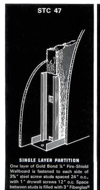
Insulation, friction fit in stud cavity.
