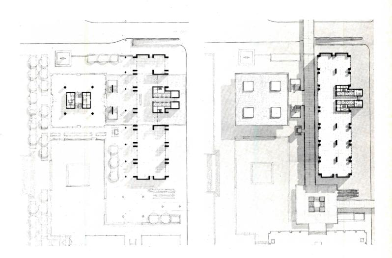
The Area 12 Building at the Charles Center in Baltimore will stand at the point of connection between the upper and lower walkway systems. The main entrance level, shown in the plan above left, if part of the lower system, with pedestrians brought down from the walkway, above right, by a double stairway. The plot plan at left shows the building's complicated relationship to other independently conceived de-
