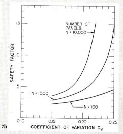
in the coefficient of variation do not have much effect, but with many lights, differences are great. With a high Cv and a large number of lights, the safety factor becomes very high. Probability of no breakage in 50 years in figure 7a is 0.667; in 7b, 0.90.
