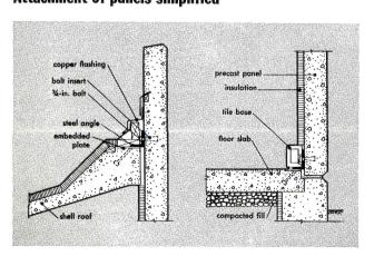
Panels were fastened to roof edge beams and the floor by bolting to steel angles which were welded to embedded metal plates. Inserts to receive ¾-in. bolts were incorporated into panels before casting. This made connections simple and expedient. And panels can easily be detached and relocated whenever plant expansion is called for.
