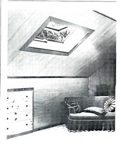
ROOF WINDOW / A leak-proof unit is insulated and provides both light and ventilation. The base is a high-density overlaid plywood. Inner and outer bubbles of the clear acrylic-plastic double dome minimize heat transmission. ■ Georgia-Pacific, Portland, Ore.
