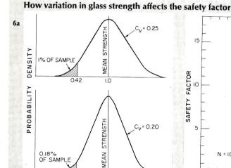
The two probability curves above illustrate the implications of the coefficient of variation, Cv. In the top curve for which the Cv=0.25, one out of 100 lights of glass would have a strength 42 per cent less than the mean. In the bottom curve, for which the Cv=0.20, only 1.8
