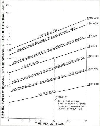
of glass strength (coefficient of variation  $C_v$ ) on these same factors. Less variability has been assumed in figure 1b ( $C_v$ =0.23) than in figure 1a ( $C_v$ =0.25).
