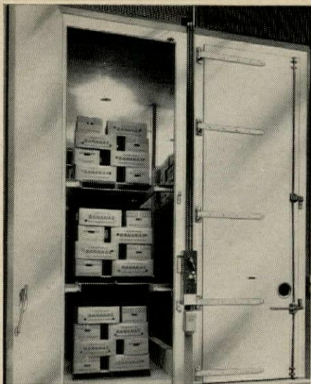
Jamison all-metal banana room doors maintain critical temperature levels and also provide gasketed seal to contain gases used in fruit ripening.
