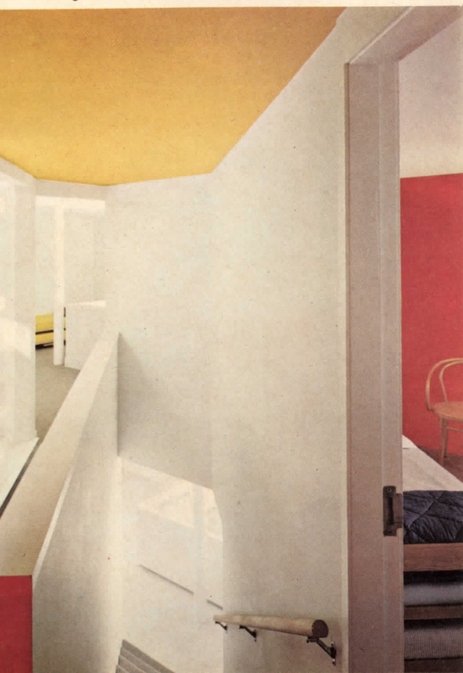
Taking in a view over the skylit, two-story breakfast space, the upstairs hall of the Hoffman house doubles back to a playroom-study for a privileged outlook and shared clerestory light. The wood frame structure is supplemented by occasional steel columns, and the subfloors are plywood or concrete slab on grade.
