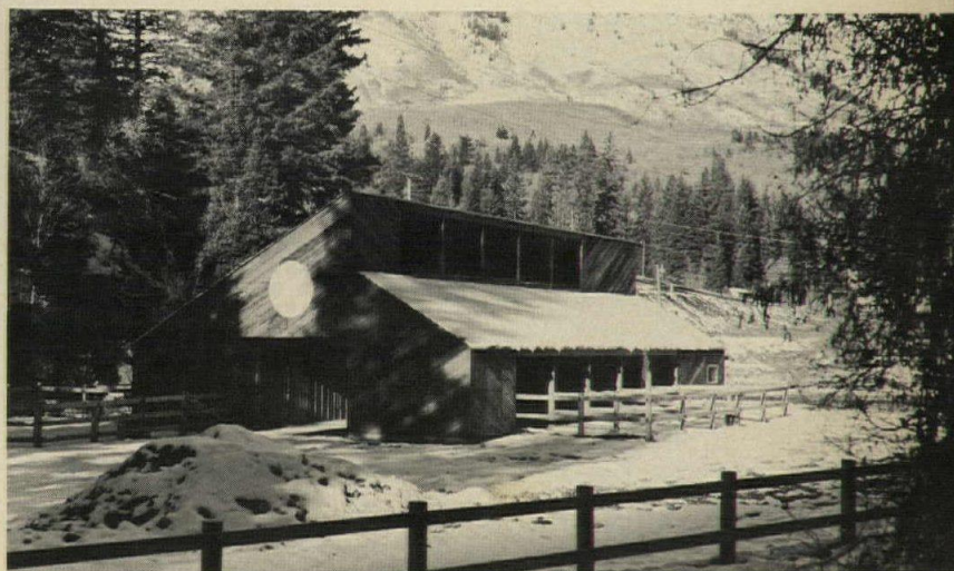
Stables for Sundance Resort , Provo Canyon, Utah, Brixen and Christopher, architects, has diagonal cedar siding and cedar roof shingles. Cost: $3.33 per square foot.
