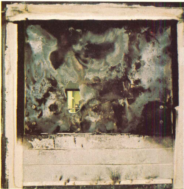
▲ Furnace fire comparison test at the U.S.G. Research Center resulted in complete disintegration of polyurethane foam insulation within five minutes.
