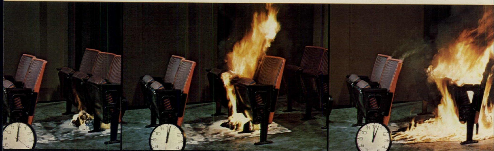
TEST TWO: HR POLYURETHANE containing flame retardants. Time: 20 seconds after ignition.
