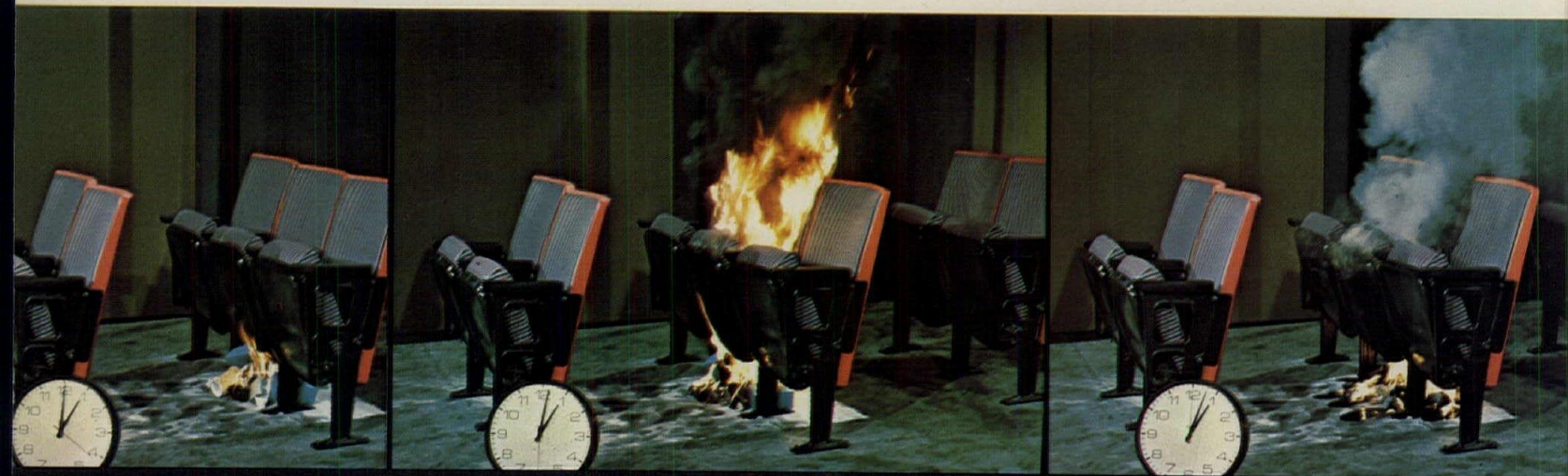
TEST ONE: DU PONT NEOPRENE Time: 20 seconds after ignition.
