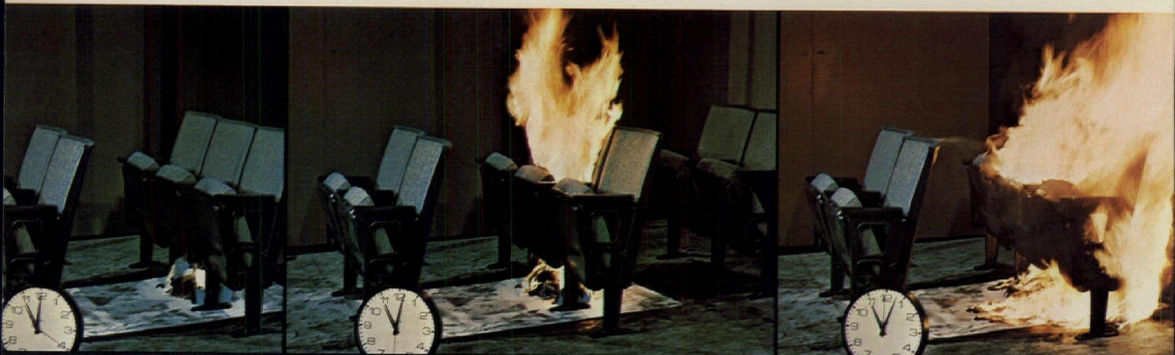
TEST THREE: STANDARD POLYURETHANE Time: 20 seconds after ignition.
