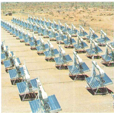
Intensive testing (EMMAQUA) conducted by Desert Sunshine Exposure Tests, Inc. in the Arizona desert has established the excellent resistance of Galbestos to color change and fade.
