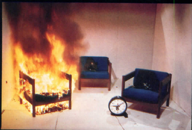
Time: 8 minutes, 30 seconds. Chairs with VONAR 3 are out. Chairs used for this test commercially available from Thonet Industries, Inc.
