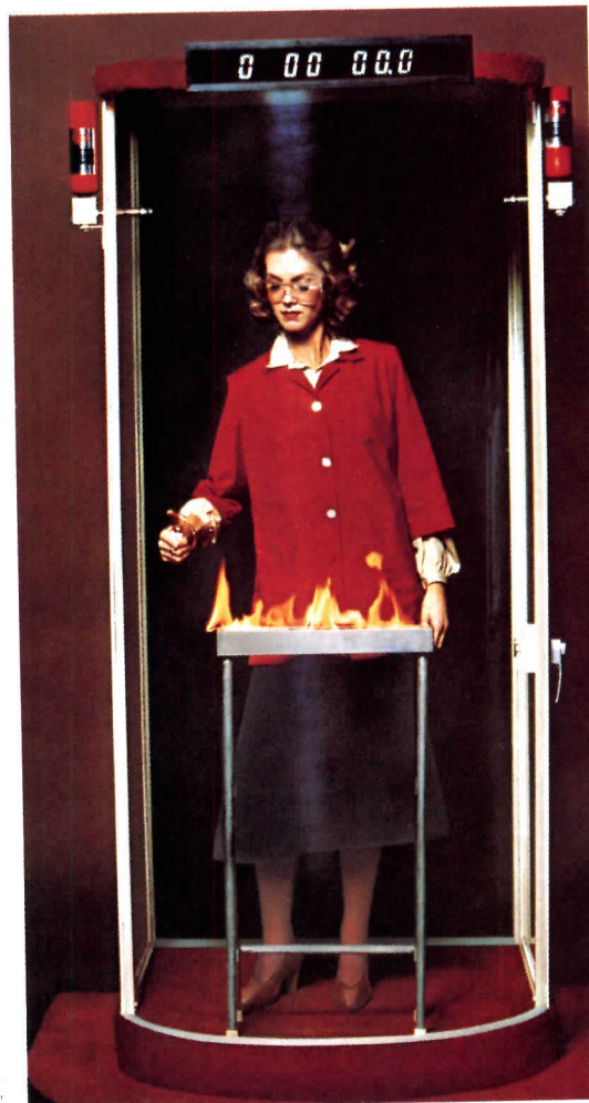
1. Flammable liquid ignited. Halon 1301 cylinders discharged.
