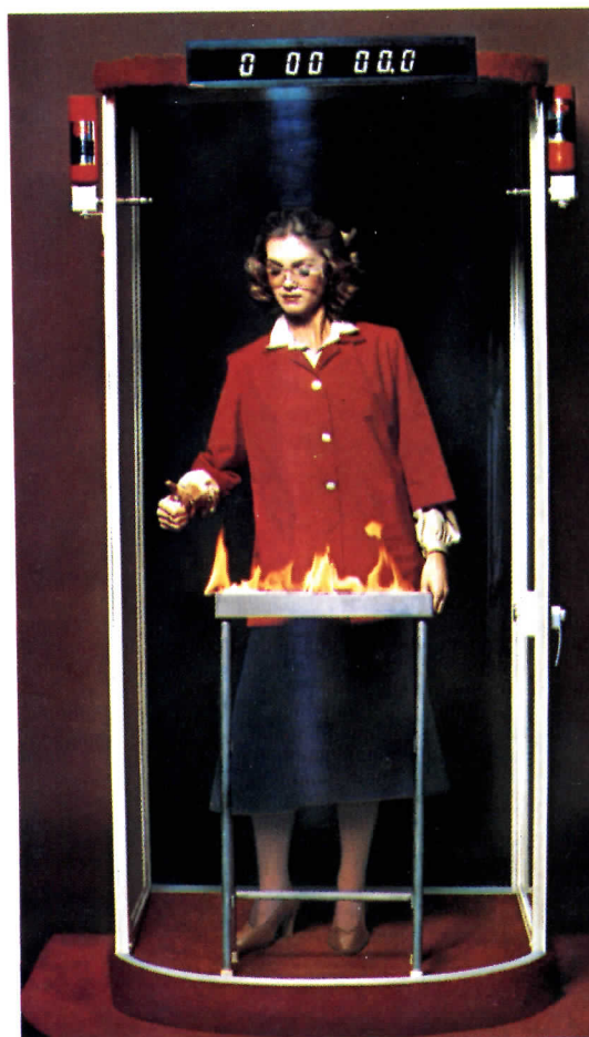
1. Flammable liquid ignited. Halon 1301 cylinders discharged.
