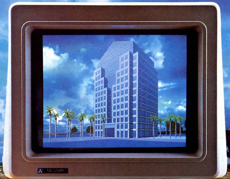
Actual images displayed on a CalComp System 25, showing rendered perspective composites onto a photographic background.
