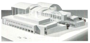
Smaller masonry-clad exhibit areas are to cluster around a series of thin metal-deck shells supported by spidery trusses at the 120,000-square-foot Virginia Air and Space Center/Hampton Roads History Center. The high, vaulted spaces will exhibit aircraft and space vehicles
