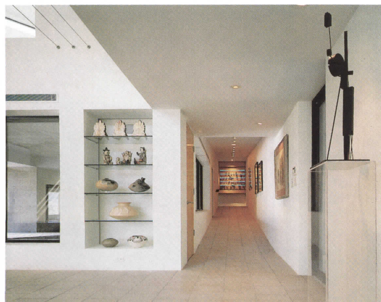
Low-voltage wires provide a flexible lighting system for the Zubers' varied collection of paintings and artifacts.
