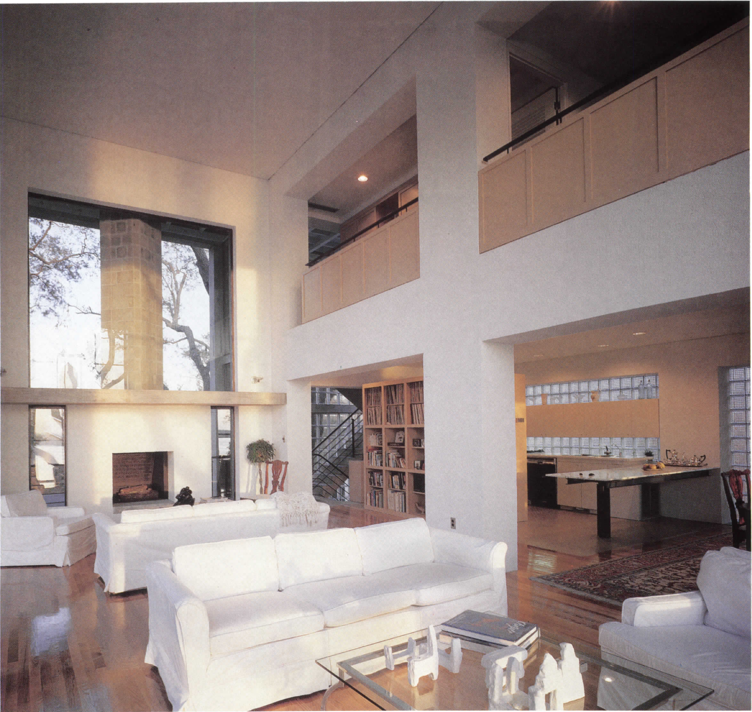
The plan of the Croffead House is organized around a single masonry pier that separates a 19-foot-high living space (left in photo above) from the low-ceilinged dining room, kitchen, and master-bedroom loft. In contrast to the severity of the concrete-block main structure, a poured-concrete stair tower (opposite) is softened by clear-glass end walls and a facade sheathed in 12-inch glass block.
