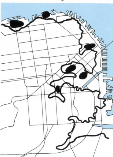
Damage concentrations within unstable areas.
