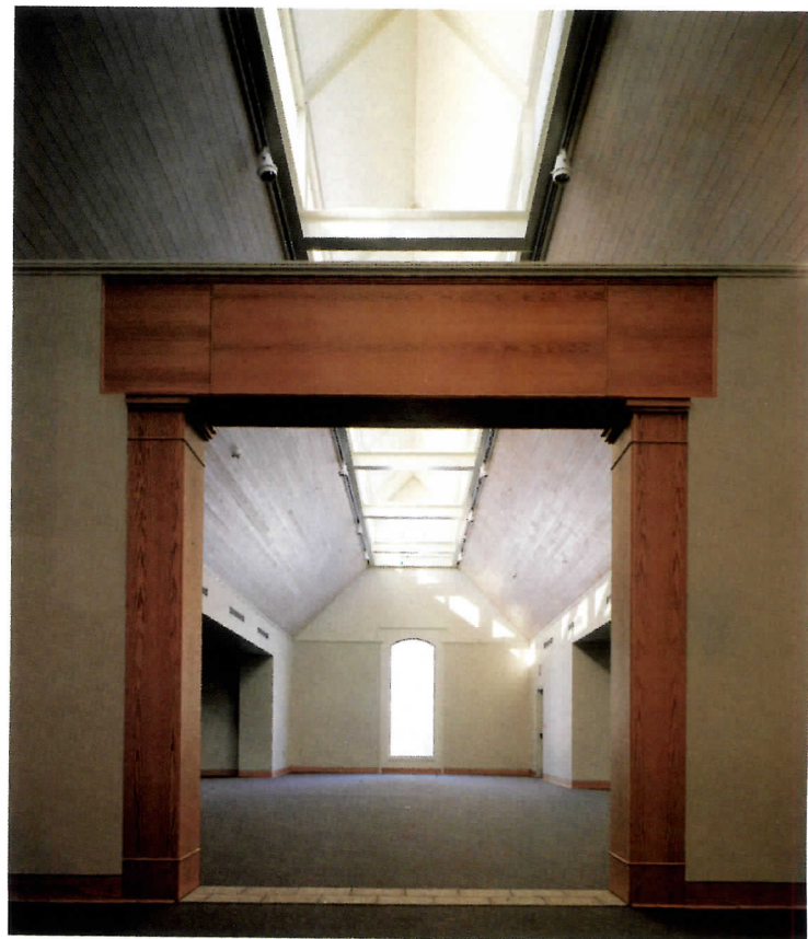
Three exhibition galleries feature clerestory daylighting.
