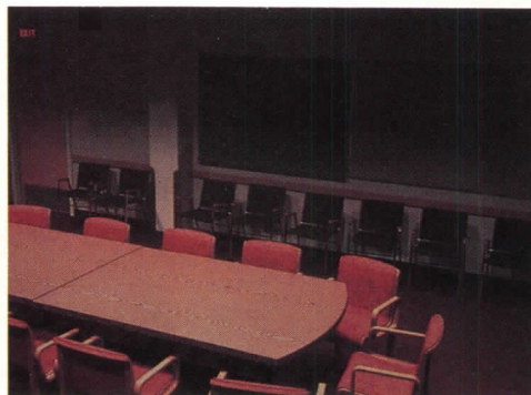
To calculate reflected light, the Radiance lighting program uses ray tracing combined with light diffusion for realistic renditions of rooms. At bottom is the computer-generated model of the actual office (top).
