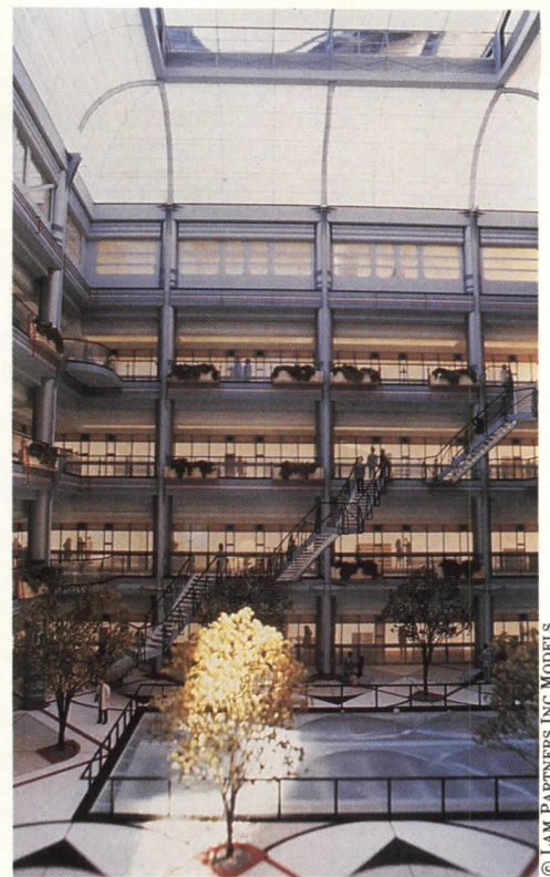
An elaborate presentation model of an atrium by Zeidler/Roberts shows more detail than most daylighting models. Though not intended for daylighting studies, it can simulate sun penetration, including the effects of a tracking roof-top mirror.
