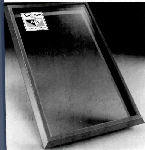
14. Low-profile skylight. Andersen Windows is now making a skylight designed to let in the most light and no water. The narrow frame installs with aluminum step-flashing and without exposed screws; units are sized to fit within American roof-construction dimensions. Glass edges are deeply captured within the sash to make condensation less likely. Andersen Windows, Inc.
