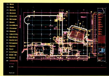
First floor plan showing colored lines that translate into varied line widths on prints.
