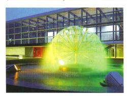
luminaires from the firm's own product line, the Martin Exterior 600 color changers. The fixtures—which the manufacturer says are durable enough to have withstood the typical sub-zero temperatures of Scandinavia, and an atypical Scandinavian hurricane as well—house a CMY color-mixing system and
