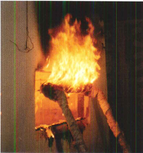
Figure 2. The photo illustrates testing in accordance with UBC Standard 26-9. The test replicates a two story structure with a fire in an interior compartment and examines lateral and vertical flame spread. The test is one of many criteria set forth in model codes to evaluate the performance of foam plastic-based wall assemblies. It is one of a series of fire tests that qualifies EIFS for use on buildings of noncombustible construction.
