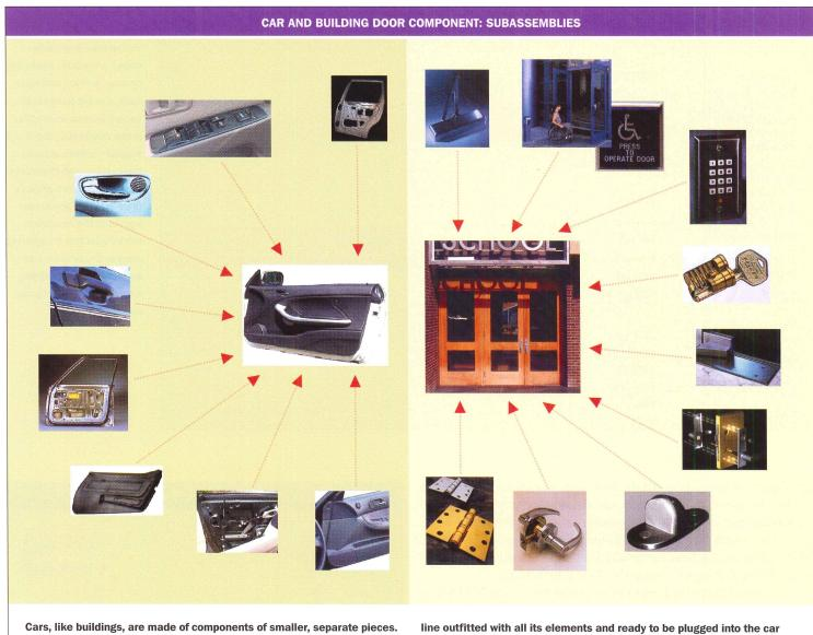
Until recently, automobile production involved installing individual parts on an assembly line one at a time. Now, the industry has shifted to a modular system in which the car door, for instance, arrives at the assembly
