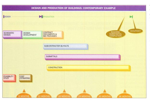
This chart (left) describes the linear process that governs the design and construction of most buildings. Almost all systems are constructed piece by piece in the field. By contrast, in a modular assembly system used by the automotive and aerospace industries (opposite, top), manufacturers use outsourced suppliers to assemble entire modules and deliver them to the factory (or building site) ready to be installed.
