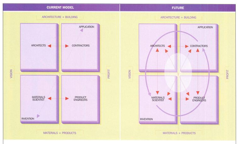
The diagram on the left shows how even in a design-build or fast-track project, the design and construction process is still achieved laterally. In their research, Kieran and Timberlake argue that there is a need for a more fluid process with more direct contributions from product
