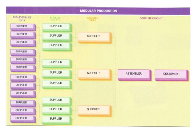
For the curtain wall at Levine Hall, Kieran **Timberlake Architects** chose a modular assembly system. In this particular case, the customer is the university; the assembler is the contractor; the Tier 1 supplier is Permasteelisa, the curtain-wall fabricator: Tier 1.5 suppliers provide the glass, the low-e coatings, and the aluminum extrusions; Tier 2 suppliers provide the interior and exterior coatings, blinds, hardware, and electronic controllers.
