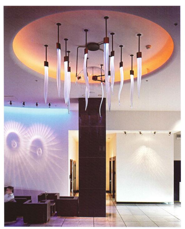
A chandelier composed of blown-glass spikes is internally illuminated by fiber-optic elements that change color (left). The ceiling cove is lit by additional low-voltage strip lights. Guest rooms feature lighting projections above each bed (below). The effect is wired on its own circuit and may be turned off separately by guests. Bedside and desk lamps designed by Piippo employ 60-watt incandescent lamps.
