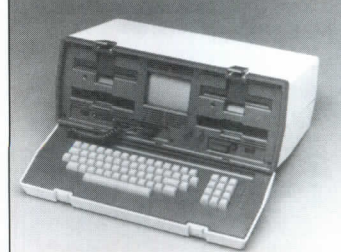
1981 Adam Osborne built the first portable computer, the Osborne I. It cost $1,795 and weighed 24 pounds.
