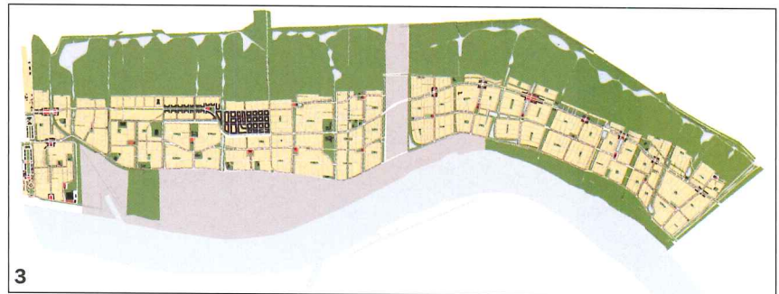
A land-banking scheme proposed by a team working in St. Bernard Parish would rebuild first in the higher, southern areas (3), moving north (2, 1) as the population grows.
