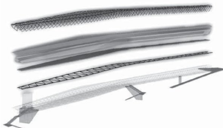
MUSEUM OF FLIGHT BRIDGE - EXPLODED AXONOMETRIC
