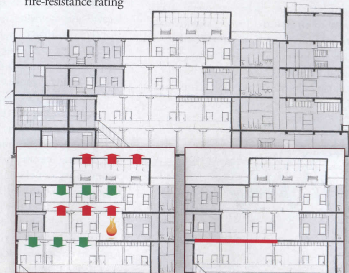
Top: Cross-sectional view of office showing offset configuration of floor openings; Bottom left: Smoke exhaust control system design; Bottom right: Horizontal flexible smoke curtain at second floor
