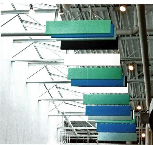
Left: Sound reverberation can be controlled with ceiling systems that are both acoustically efficient and visually exciting. Right: Vertical acoustical treatments such as baffles used in this ceiling space help to control reverberation time and overall sound quality.
