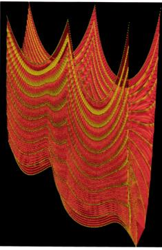
Engineers from Buro Happold created a finite-element-analysis model of Air Garden. An axonometric view (left) created from this model. reveals the amount and complexity of the data that was analyzed. Among the studies that the engineers performed for Ball-Nogues was an examination of the forces acting on the bead chains (far left). Stress increases near the supports, since the uppermost sections of the bead chains must carry the weight of those below
