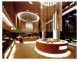
Using hardwood slats to build architectural elements may not be an option due to weight or cost. But B+N Industries has developed a system that replicates them, using aluminum covered in a non-PVC surface. Reducing weight, waste, and cost, it can be used as walls, ceilings, screens, handrails, and more, in both interior and exterior environments. bnind.com circle 201
