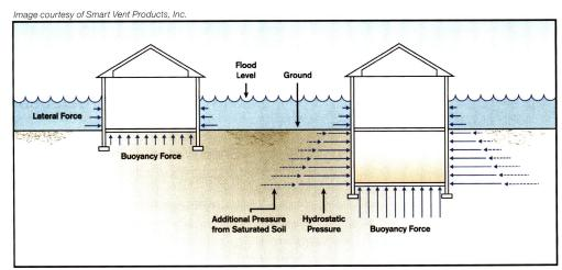
Design professionals who understand the forces at work in an extreme environmental situation, such as flooding, can appropriately create buildings that can tolerate stresses and recover quickly.
