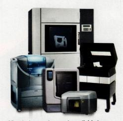
3D printing equipment is available in a variety of sizes for a variety of needs using different types of materials that can make architectural models.
