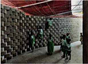
After laying stone, used for seating rings (above and right), proved too timeconsuming, the team made concrete blocks on-site for walls (left). Shadows cast by the blocks' projecting corners cut heat loads. Overlapping roof planes (opposite) promote ventilation, and adjustable fasteners permit movement in any direction for struts.
